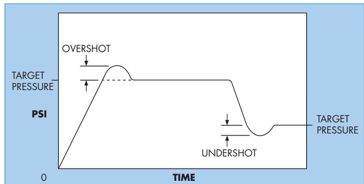
The PPC is based on a closed loop design which combined with MACs fast responding, very repeatable, high flow, balanced 2-way valves, optimizes response and accuracy, practically eliminating overshoot and undershoot.
