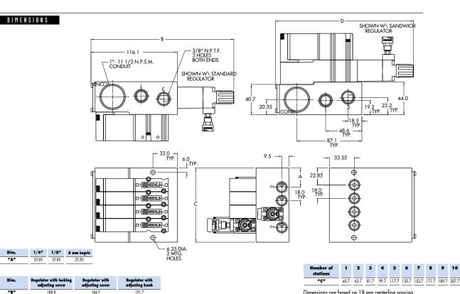
Dimensions are based on 18 mm centerline spacing Note: Bottom & side cylinder ports not available on the same station
