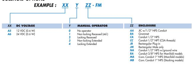
(MA & MB common conduit covers require 1#M-01002-01 conduit end plate kit per stack)
