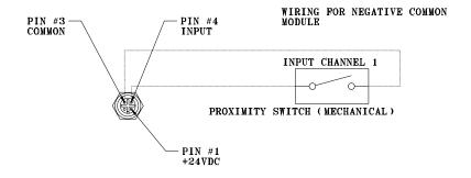
NOTE, FOR ELECTRONIC SWITCHES, CONSULT THE MANUFACTURER'S RECOMMENDED WIRING PROCEDURE.
