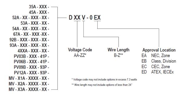
The list above represents current compatibilities with the Hazardous Locations approved D-coil. Additional series could be modified to accept a hazardous location pilot if necessary.
