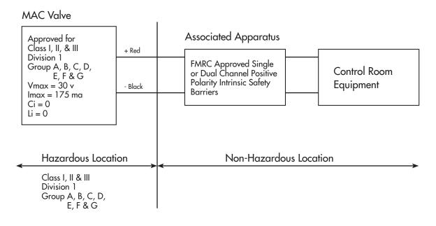
There are 3 basic parts to an intrinsically safe circuit :
