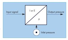
The key to the MAC PPCs are two MAC 34, 45, 400, 47, 92 or 93 Series valves that are used to control the output pressure. The valves are operated by the PPCs closed loop electronic control circuit. Feedback is obtained from one or two transducers. The balanced poppet, fast response, and high flow of these two MAC Valves provide outstanding performance characteristics for the PPC.
