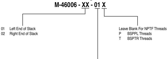
Note: "01" should be used only when the Fastening End Plate Kit is ordered separately. When the kit is ordered with an assembly this number will change to indicate the number of <u>valves</u> in the stack.
